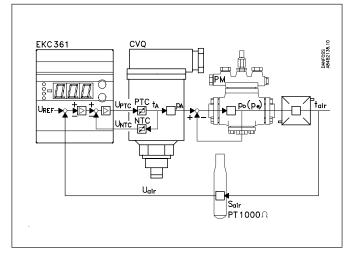
The allowed temperature in the actuator determines the evaporating pressure Actuator temperature °C ANFOSS 84B2139. 140 130 CVQ 0—≻6ba 120 110 100 90 80 70 60 50 40 5 0 2 3 4 6 7 p bar eff -100 - 26 - 10 1 9 16 22 32 to °C R134a 26 -100 -41 -25 -14 -6 0 16 to °C R22 6 11 -100 -34 -19 -9 -2 4 9 13 17 to °C R717
