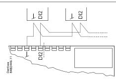
The following controllers can be connected in this manner: EKC 202D /302D series and AK-CC 210 and AK-CC 250 Max. 15
