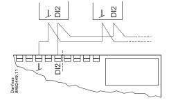
The following controllers can be connected in this manner: EKC 202D/302D serie and AK-CC 210 and AK-CC 250 (But max. 15 controllers)
