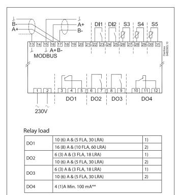
DO1 is 20 A relay. DO2 and DO3 are 16 A relays. DO4 is a 10 A relay. The max. load listed above must be observed when connecting without zero-crossing control. When connecting with zero-crossing control, the load must be increased to the value indicated by 2)
