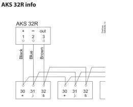
The signal from one pressure transmitter can be received by up to ten controllers.
