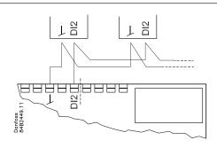
The following controllers can be connected in this manner: EKC 202D /302D serie and AK-CC 210 and AK-CC 250 (max. 15)
