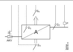
Evaporator control with one to four evaporators
