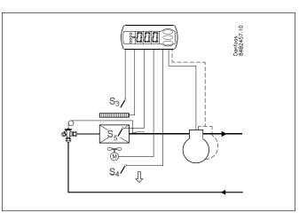
Controller with four relay outputs, three temperature sensors and two digital inputs.
