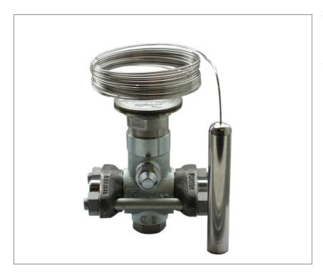
Thermostatic expansion valves regulate the injection of refrigerant liquid into evaporators. Injection is controlled by the refrigerant superheat.
