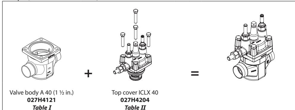
*ICV 40 valve body w/different connections*
