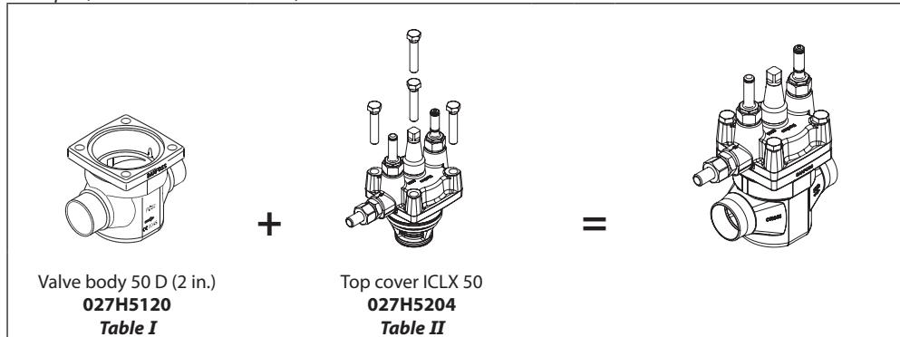
ICV 50 valve body w/different connections
